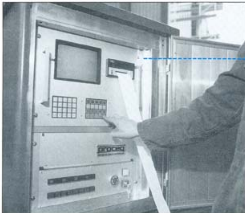
The weighing results are instantly monitored and printed.
